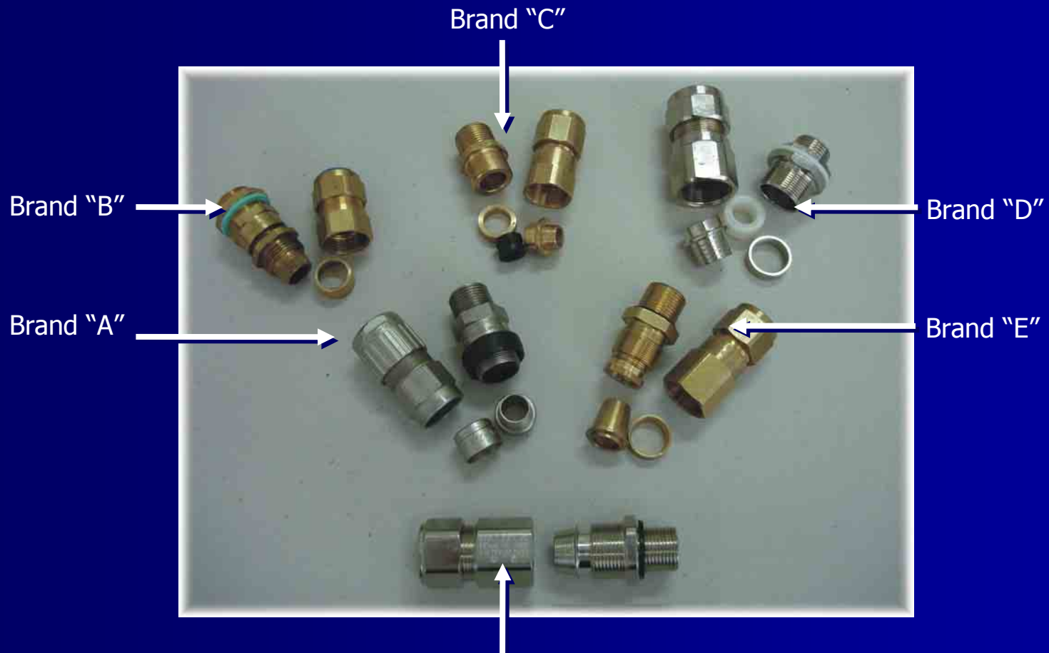
CCG with captive components
